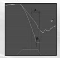
Here is an example of where well judged variation of pressure on the brake pedal (part D) results in a significant time gain. Slipping (part C) has been reduced to a minimum and the wheels did not block.
